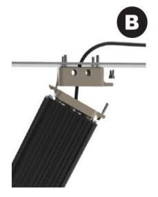
Step 2 - Attach the lamp body to the top of the junction box under the lid of the junction box. (Figure B)
