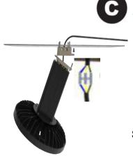
Step 3 - Connect the L,N,GND wires on the lamp to the corresponding L,N,GND cables on the pole. (Figure C)
